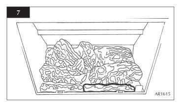
7.7 Place log E across from the rear of log A to log C on the right hand side. Again, there are cut-outs for location. The front of the log should sit on the front ash panels and should fit tight to log C. See diagram 8.
